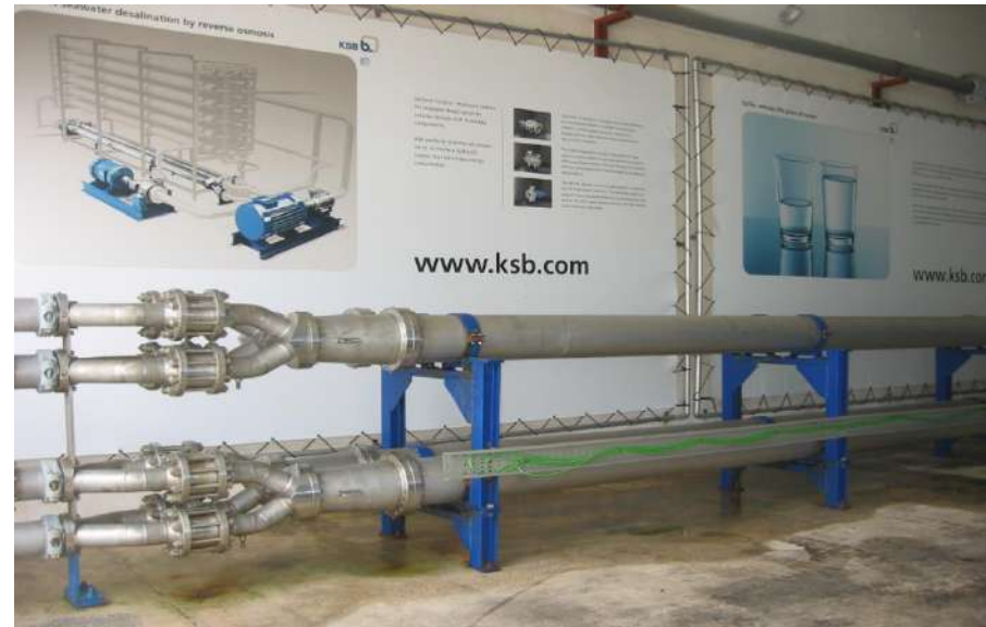
← Testing 16 inch membrane elements for Toray
