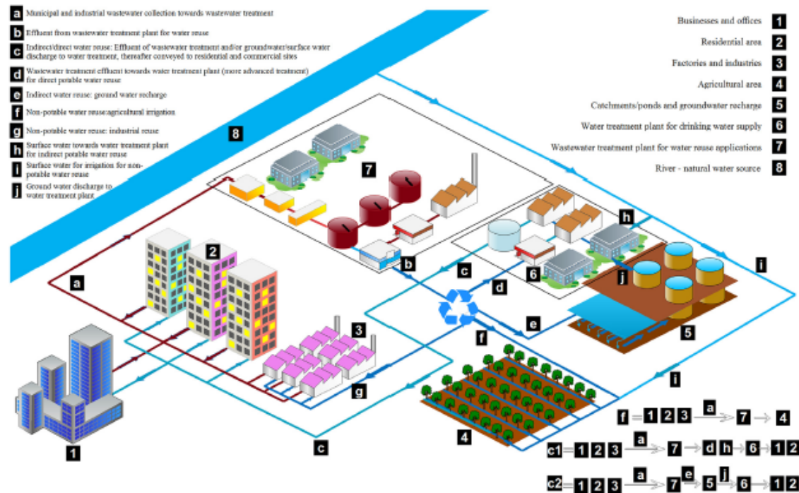
Fig. 2. Illustration of the different possible water reuse applications within a community.
